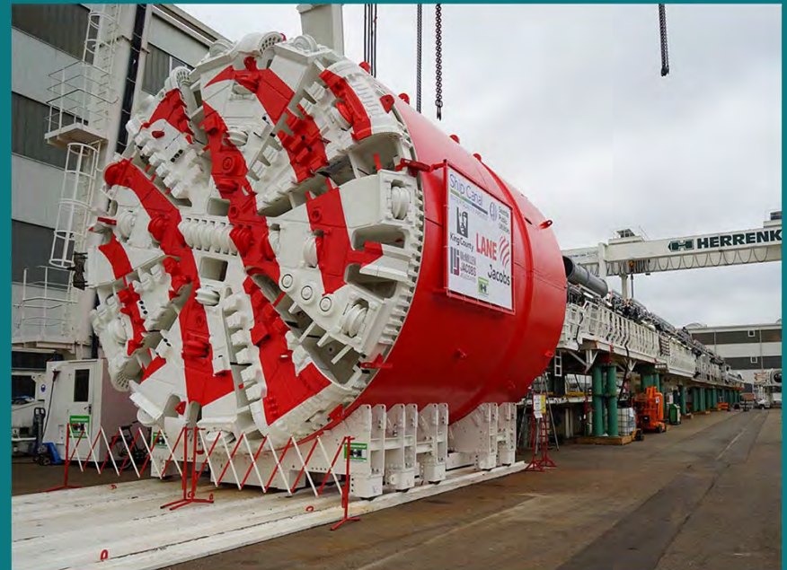
Example EPB TBM for 18-ft finished diameter tunnel – Seattle Ship Canal Water Quality Project
